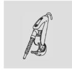
2. Plug the programming plug into the socket. Use the programming cable CS-44 A (Phonak version) only. Key features
