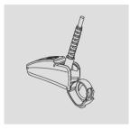
2. Plug the programming plug into the socket.
